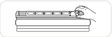
Change the batteries and tip headrail back into place.
